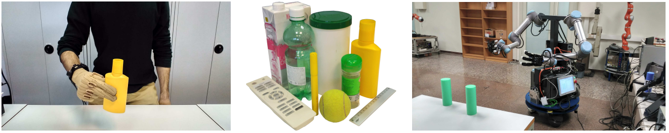
Fig. 1. Human operator wearing the measurement equipment (left), set of objects used in the experiments (middle), and dual-arm robot (right).
