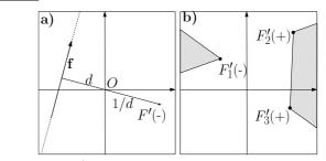
Figure 4: a) A force **f** and its dual representation F'b) Linear combination of three dual forces, one of them with different sign from the others.
