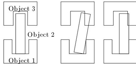
Figure 1: *Advantages and disadvantages of the clearance in a three object assembly.*
