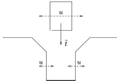
Figure 2: *Assembly direction ( $\hat{t}$ ) and uncertainties increasing the difficulty of the task ( $u$ ).*
