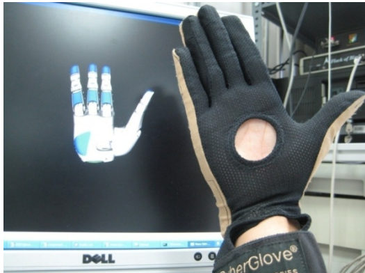
Fig. 1 Human hand with the sensorized glove connected to the mechanical hand simulator used in the data acquisition procedure. This is the “0” configuration, which means all the joint angles are 0 in this configuration.
