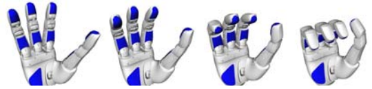
Fig. 2. Configurations of the SAH hand when it is moved along the first PMD (i.e. with only one DOF). Reproduced from [21].
