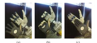
Fig. 14: Poses performed wearing the data glove and then sent to the robotic hand.
