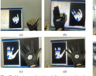
**Fig. 13:** Mapping results. (a) and (b) correspond to the fingers flexion movement, (c) and (d) correspond to the fingers abduction movement.
