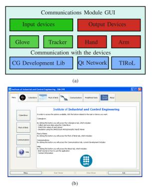
**Fig. 9:** Communications Module. (a) Module structure, input devices are access through the CyberGlove development library and output devices using a client-server based model, (b) Developed graphical user interface.
