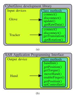
**Fig. 7:** C++ object definition. Integration of the devices is done using the proprietary software libraries as part of the application, in order to access their features.
