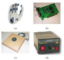
Fig. 5: Robotic hand system. (a) Robotic hand, (b) PCI card, (c) Mounting base, (d) Power supply.
