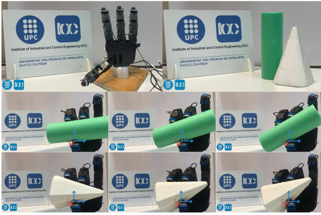
Fig. 3: First row left: Allegro hand equipped with the Optoforce tactile sensors. First row right: the objects manipulated during the experiment. Second and third rows: Different sequences of the reorientation, in the x -axis of the reference frame, of the grasped object.
