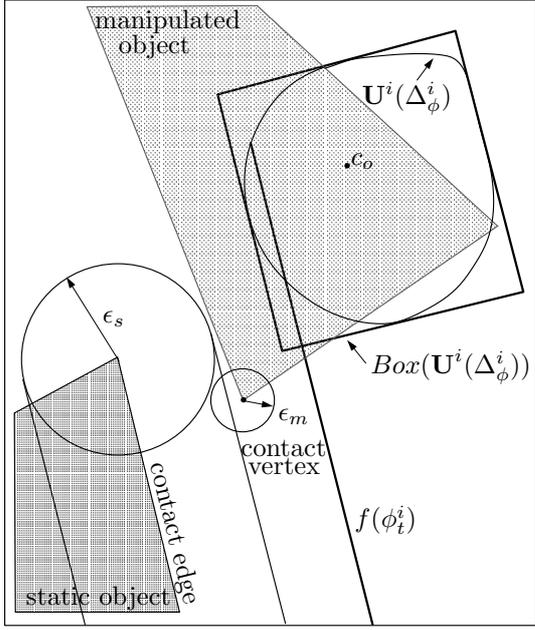
Fig. 1. *Single-contact identification.*
