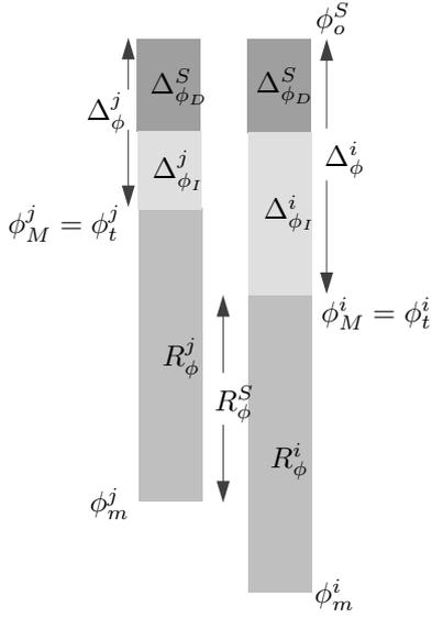
Fig. 2. Ranges of nominal contact orientations ( $R_\phi^i$ ,  $R_\phi^j$  and  $R_\phi^S$ ) and signed distances  $\Delta_\phi^i$  and  $\Delta_\phi^j$  from  $\phi_o^S$  to  $R_\phi^i$  and  $R_\phi^j$ , respectively which are due to both dependent and independent sources of uncertainty.
