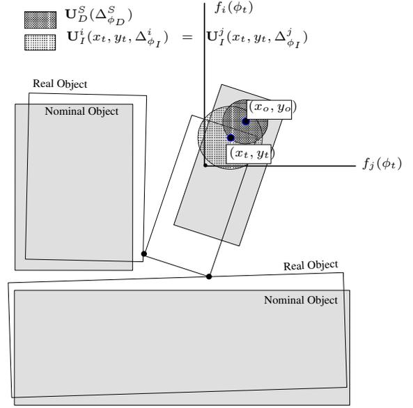
Fig. 3. Effect of dependent and independent sources of uncertainty: The current configuration of the manipulation object is at a possible contact configuration of a nominal two-basic contact situation, since  $\mathbf{U}_I^i(x_t, y_t, \Delta_{\phi_I}^i) \cap f_i(\phi_t^i) \neq \emptyset$  and  $\mathbf{U}_I^j(x_t, y_t, \Delta_{\phi_I}^j) \cap f_j(\phi_t^j) \neq \emptyset$ .
