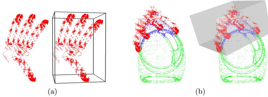
**Fig. 3.** (a) Left:  $P_h$  representing the grasping configuration of the Allegro Hand. Right:  $MBB-P_h$  obtained for a point cloud of the Allegro Hand representing the grasping configuration. (b) Left:  $P_h$  and  $P_g$ . The red points represent the Allegro hand, the green points represent  $P_p$  and the blue points are in contact or enveloped by the hand. Right:  $MBB-P_h$  is shown in solid to show its dimension.
