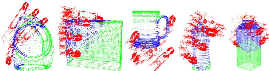
**Fig. 6.** Example of a random grasp for each object. Red points represent the grasping hand pose  $P_h$ . Green points compose the point cloud that represents the reachable part of the object  $P_p$ . Blue points are the points that are in contact or enveloped by  $MBB-P_h$ .
