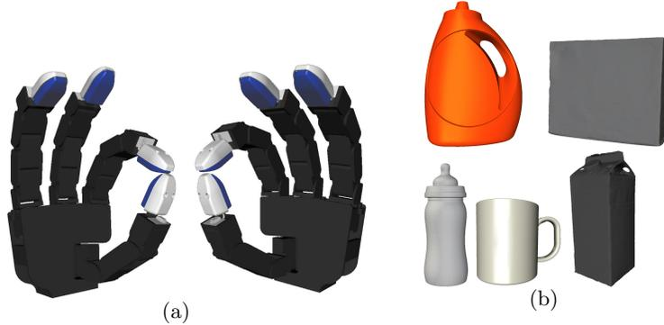
**Fig. 5.** (a) Allegro Hands. (b) Objects used for experimentation: a detergent bottle, a cookie box, a feeding bottle, a coffee mug and a milk box.
