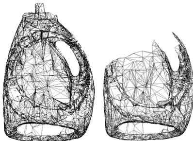
**Fig. 4.** Triangular mesh models  $M_g$  and  $M_p$  of a detergent bottle computed from  $P_g$  and  $P_p$  respectively
