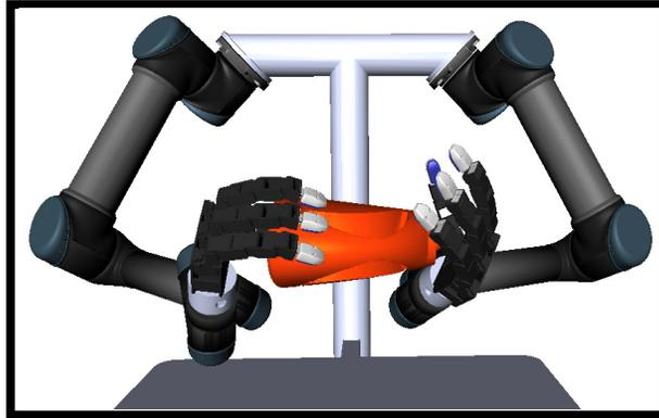
**Fig. 1.** Dual-arm robot (ADARS: Anthropomorphic Dual Arm Robotic System) about to perform a transfer of the object from the right to the left hand.
