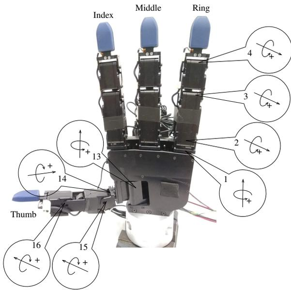
Fig. 1. Anthropomorphic robotic hand Allegro Hand, with 16 *DOF* and 4 fingertips with tactile sensors WTS-FT. Axes of rotation of the joints are indicated; the index, middle and ring fingers have the same kinematic structure. Thumb finger can rotate (abduction movement) over the hand palm.
