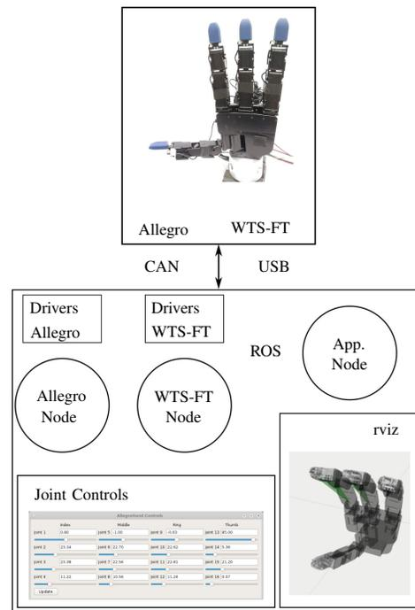
Fig. 3. Hardware and software components overview. Allegro Hand uses a CAN bus for the connection with a PC and WTS-FT sensors in the fingertips use USB. All software components are integrated using Robotic Operative System (ROS) as communications layer.
