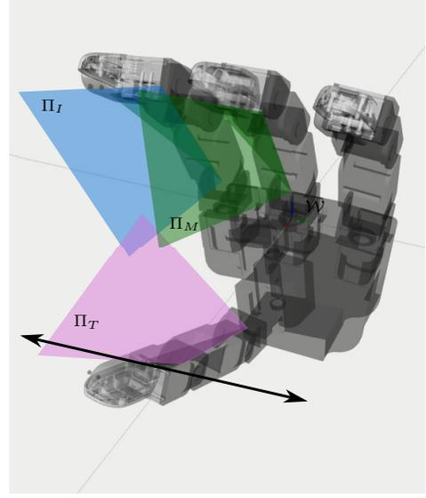
Fig. 4. Allegro hand with the finger working planes for Index, Middle and Thumb. Working planes are oriented as parallel to each other as possible, allowing the object rotation around an axis parallel to the hand palm plane.
