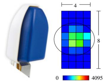
Fig. 2. Tactile sensor WTS-FT with graphical representation of a measurement highlighting with an ellipse the contact region. The bar in the bottom indicates the scale of colors corresponding to the force values returned by each texel.
