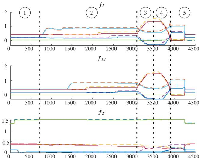
Fig. 11. Evolution of joint values (in Radians) of the three fingers while a jar with flat faces was manipulated. In dashed line, the commanded joints values. In continuous line, the reached joint values.
