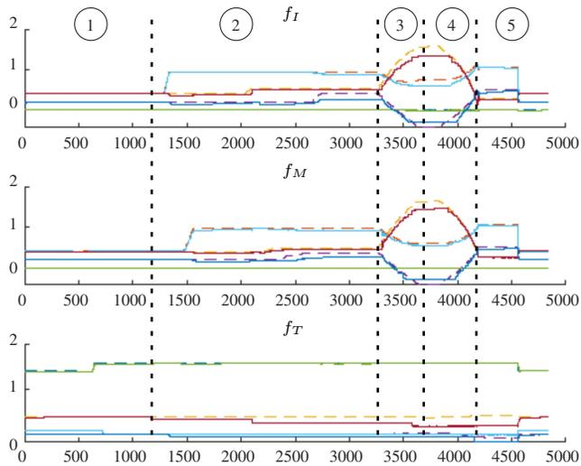
Fig. 7. Evolution of joint values (in Radians) of the three fingers while a larger regular bottle was manipulated. In dashed line, the commanded joints values. In continuous line, the reached joint values.
