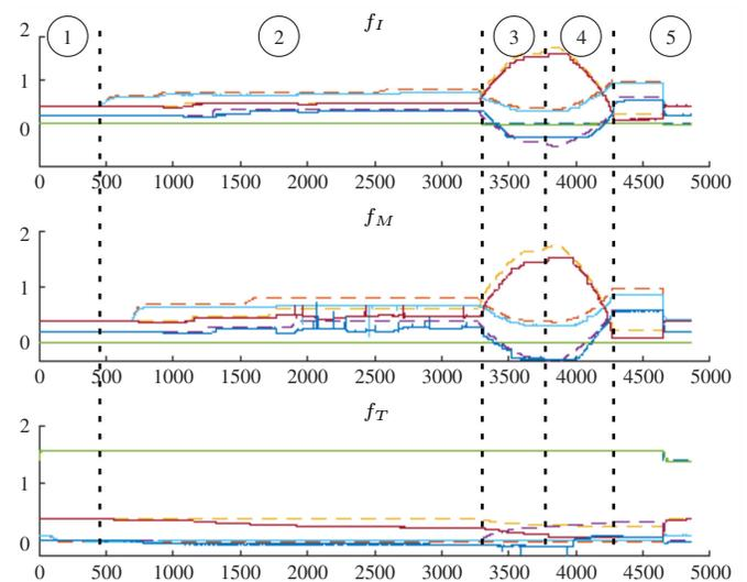
Fig. 9. Evolution of joint values (in Radians) of the three fingers while a bottle with multiple curvatures was manipulated. In dashed line, the commanded joints values. In continuous line, the reached joint values.
