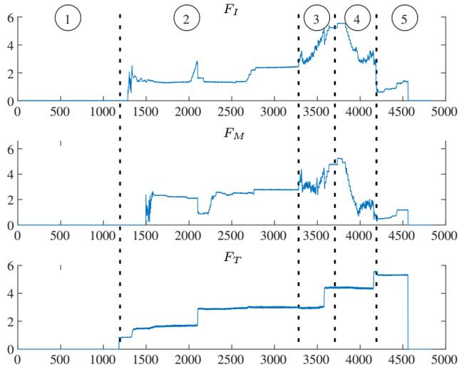
Fig. 8. Evolution of the measured forces (in Newtons) at the fingertips while a large regular bottle was manipulated.
