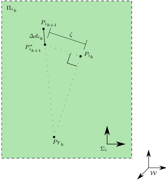
Fig. 5. Example of the computation of  $P_{i_{k+1}}$ ,  $i = \{I, M\}$ , in case that the contact force  $F_{i_k}$  is larger than  $F_{i_d}$  the target virtual contact point  $P_{i_{k+1}}$  is moved away applying the adjustment  $\Delta d_{i_k}$ . All points are projected onto  $\Pi_{i_k}$ .
