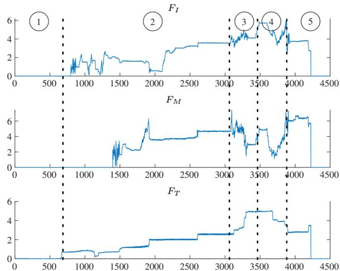
Fig. 12. Evolution of the measured forces (in Newtons) at fingertips while a jar with flat faces was manipulated.
