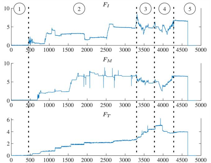
Fig. 10. Evolution of measured forces (in Newtons) at fingertips while a bottle with multiple curvatures was manipulated.
