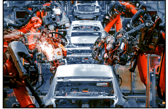
Fig. 1. Automotive BiW with several robots sharing the same workspace.
