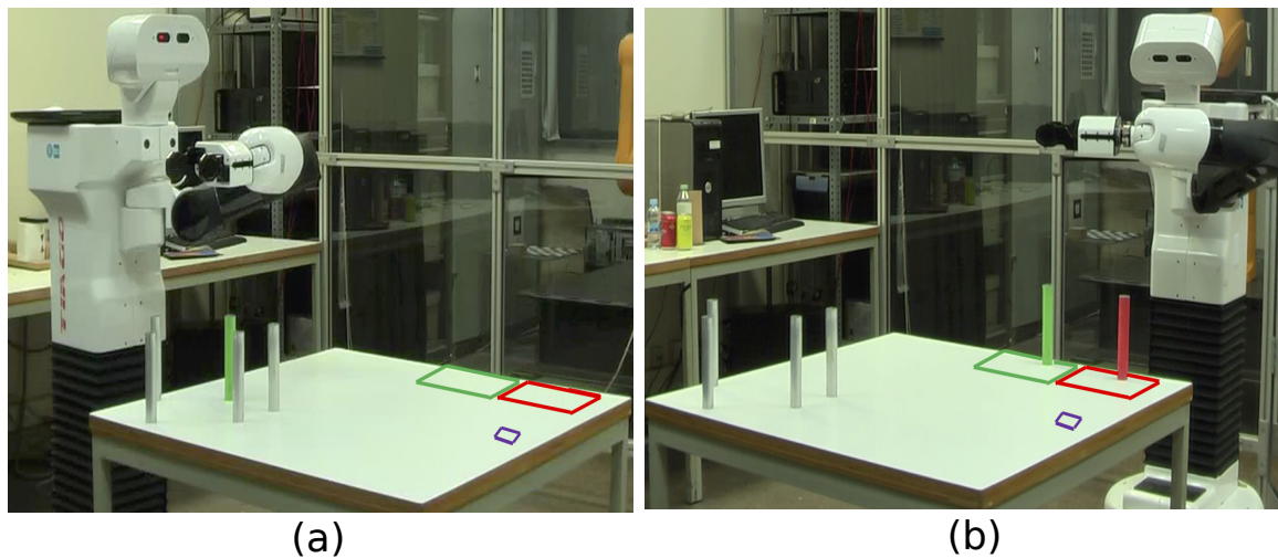
Figure 7. The manipulation example where green and red objects must be placed in the green and red regions. (a) shows the initial state of the problem. (b) shows the final state of the problem. The red object is not initially located in the robot workspace. The pink region is the place where human can transfer objects to the robot workspace. The solution can be visualized here: https://sir.upc.es/projects/ontologies/GreenRedHuman.mp4 . The solution for the case that the red object is initially located on the table is visualized here: https://sir.upc.es/projects/ontologies/TiagoRedGreenRob.mp4 .
