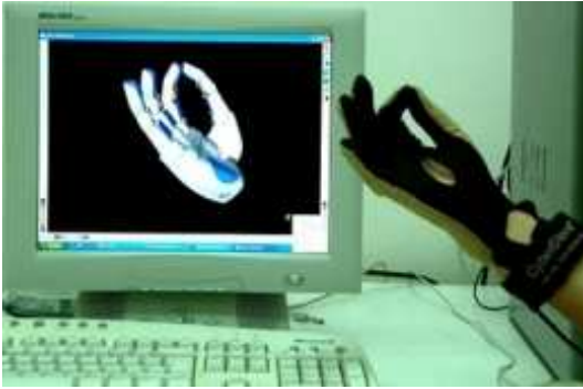
Fig. 5. Human hand with the sensorized glove connected to the mechanical hand simulator used in the data acquisition procedure.
