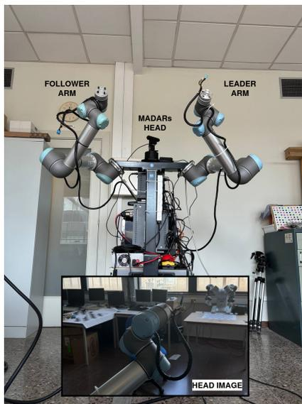
Fig. 5. Visual guidance demo: The user manipulates the leader arm and the visual guidance system tracks its end-effector (maintaining it at the center of the image) sending its frame to the other arm, that follows it with a given predefined transformation.
