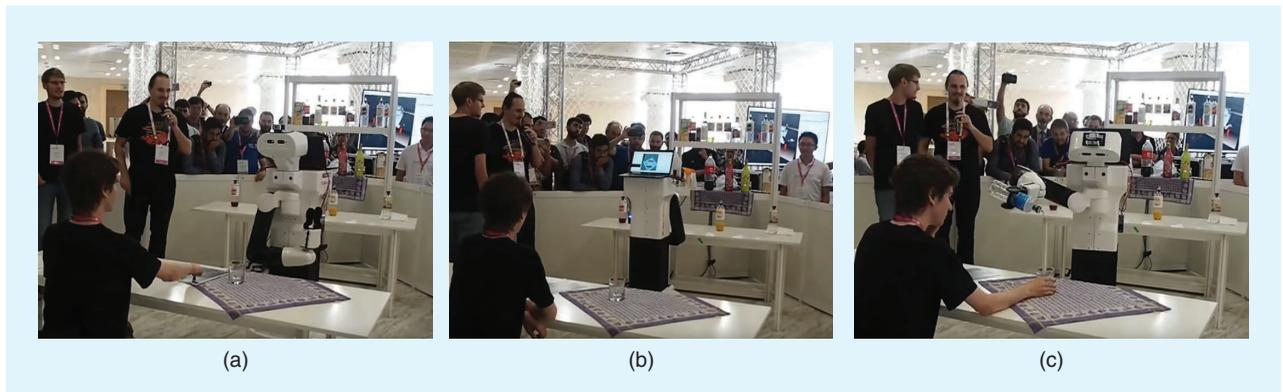
**Figure 4.** The TAMS demonstration. (a) A user points at a menu to order a drink. (b) TIAGo moves to a bar to retrieve the liquor. (c) The robot pours the (real) liquor into a glass.
