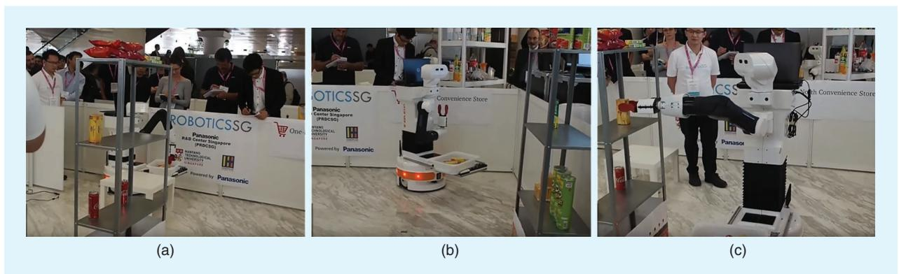
**Figure 5.** The Robotics.SG demonstration. TIAGo (a) retrieves a bin with returned items, (b) navigates a store by using a pre-recorded map, and (c) places an item on the required shelf.
