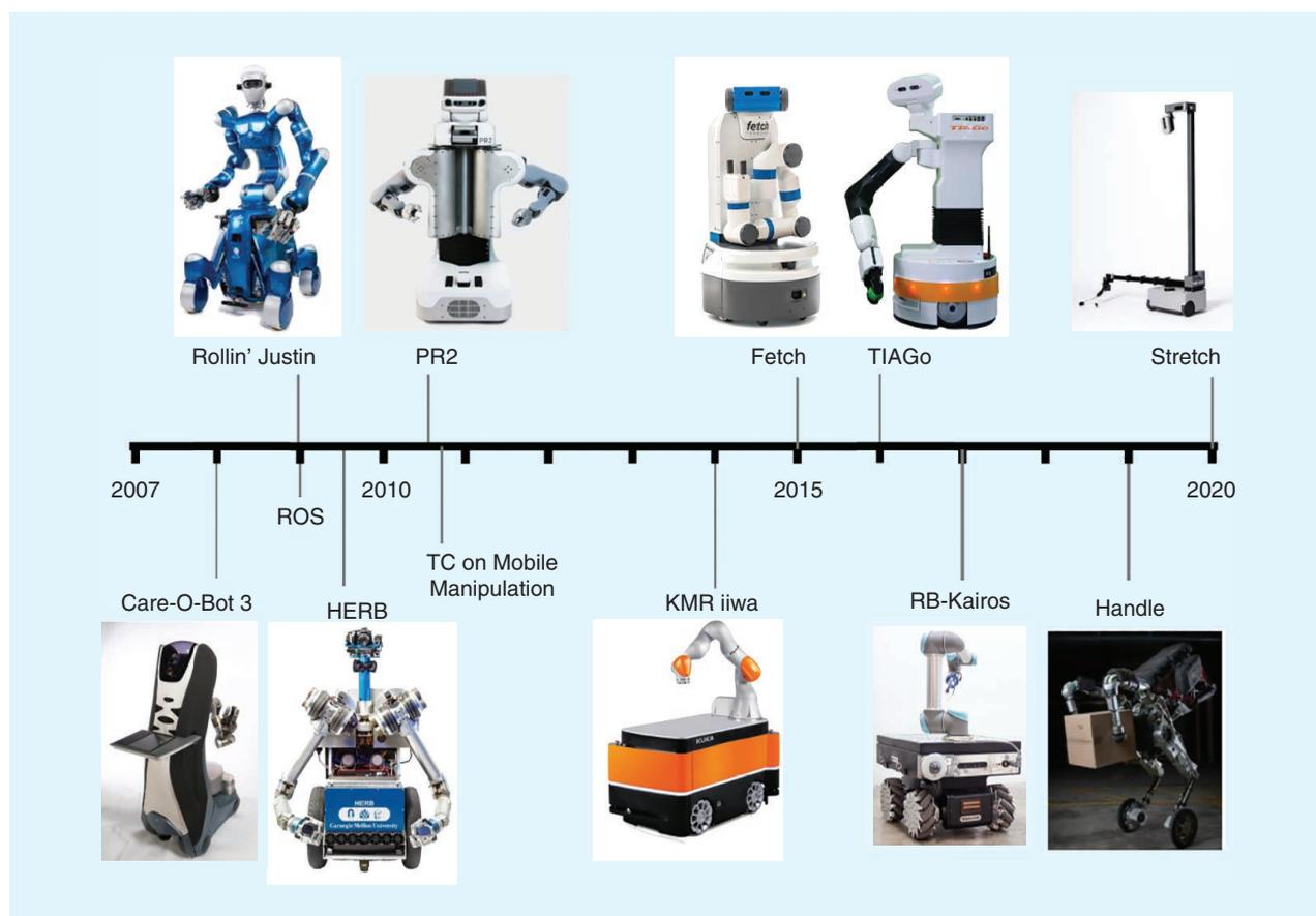
**Figure 1.** Wheeled robotic manipulator development during the past decade.
