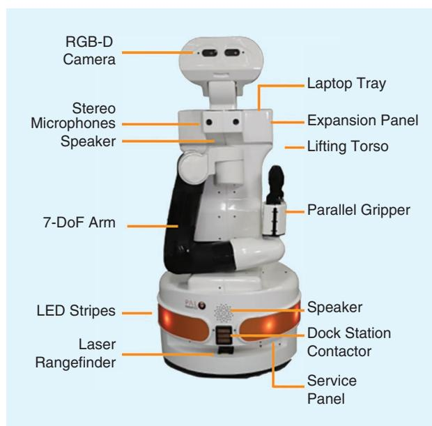
**Figure 2.** The TIAGo wheeled manipulation platform.
